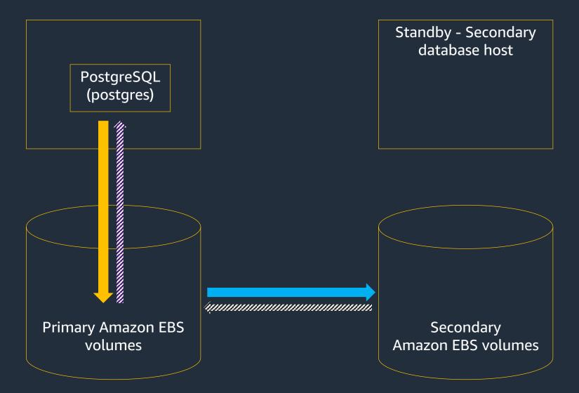
Write latency = cumulative latency of (local write + local acknowledgement) + ((remote write + remote acknowledgement))
