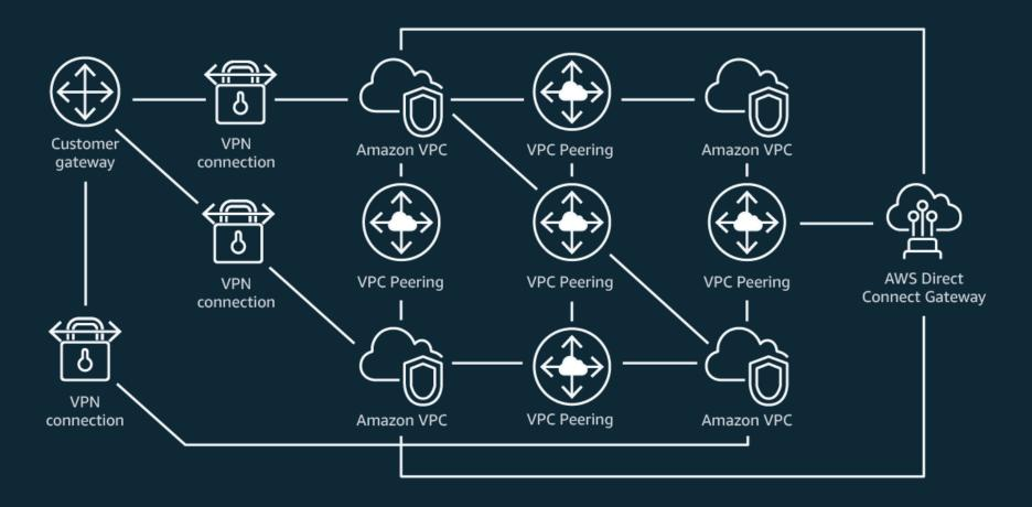
Connecting large number of VPCs in a mesh is challenging to manage
